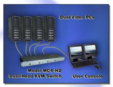
There are 3 ways the *MC4-H2* can switch from one PC to another. The first is through the buttons located on the front panel of the *MC4-H2*. The second is through a hot-key sequence from the keyboard and the third is through RS-232 control.
